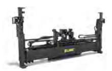
**ELME 584LD Innovation double-stacking spreader** The 584LD is an 24200-lb telescopic side lift spreader for handling two empty ISO/reefer containers simultaneously. It engages and secures the containers with two horizontal lifting hooks and side clamps. Ideal for heavy-duty double handling applications, combined with handling eccentric load, it can take double reefer containers with refrigeration units aligned. This simplifies handling and improves lifting efficiency.
